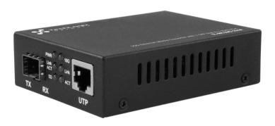
The TL-MC10G-1S1R features one SFP+ port (SFP module sold separately) and one RJ45 twisted pair port, effectively adapting twisted pair-based devices to fiber for longer transmission distances. The TL-MC10G-1S1R supports multimode fiber when paired with a multimode SFP+ module and single mode fiber when paired with a single mode SFP+ module.
