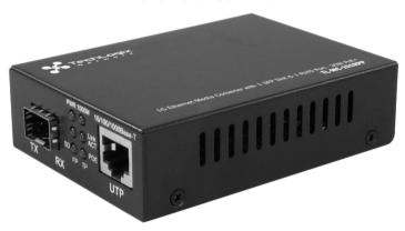
The TL-MC-1S1RPP features one SFP port (SFP module sold separately) and one RJ45 twisted pair PoE+ port, effectively adapting PoE and PoE+ twisted pair-based devices to fiber for longer transmission distances. The TL-MC-1S1RPP supports multimode fiber when paired with a multimode SFP module and single mode when paired with a single mode SFP module.
