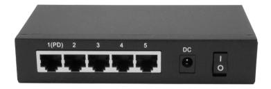
The TL-NS5R-POE is equipped with five Gigabit ports, a power connector and an on/off switch. Each of the four PSE ports (Ports 2-5) can provide up to 30 watts. The product is compliant with IEEE 802.3af and IEEE 802.3at standards and can be powered either by the included adapter or via PoE.
