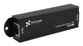
The ENET TL-PE-30W is designed to extend connection distances from a PoE source to an output device another 100 m (328 ft.) via twisted pair cable. You can cover even longer distances by cascading these extenders on a network. The TL-PE-30W does not need any additional power supply, as it draws the power it needs from the PoE input.
