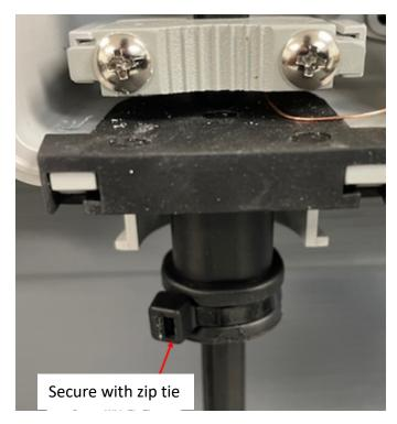
2. Use the variable cable entry clamp to secure the incoming fiber cable.
