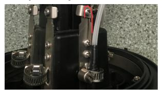
3. Remove the sheath of the cable and clean it. Cut the strengthen member to 5cm length. Put it through the attach screws and bend it to fix on the screw. Then tighten the screw.
