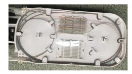
6. Coiling the optic fibers in the splice trays as above picture from the bottom tray to the top one. Fusion the joints and shrink the protective tubes and fix them in the tray. Put on the tray lid.
