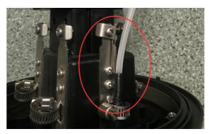
4. Remove the loose tube of the cable and clean the bare fibers. Put them through the transparent PE tube. Using PVC tape to wrap the end of the PE tube and cable.
