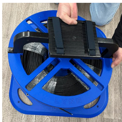
Step 7: Reattach the tray aligning the tray over the coil stops.
