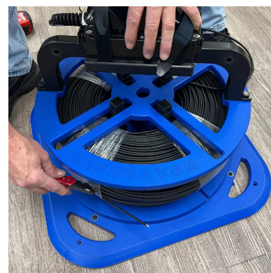
Step 9: If using on grass, install the ground stakes at each corner. Remove the stretch wrap from the coil and you are ready to unwind the coil.
