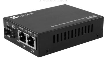
The TL-MC-1S2R features one SFP port (SFP module sold separately) and two RJ45 twisted pair port2, effectively adapting twisted pair-based devices to fiber for longer transmission distances. The TL-MC-1S2R supports multimode fiber when paired with a multimode SFP module and single mode fiber when paired with a single mode SFP module.
