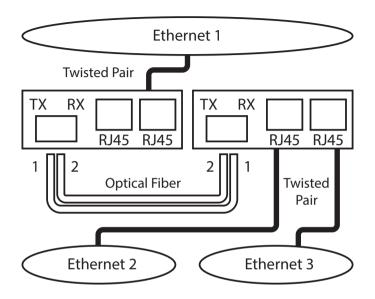
As shown above, two fiber optic cables need to be connected between two ideally identical media converters. Make a connection from Media Converter 1 TX to Media Converter 2 RX, and from Media Converter 1 RX to Media Converter 2 TX.
