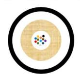
M3I-12M-P-BK fiber optic cable is constructed with twelve internal tight buffers, internal aramid yarn, and one outer plenum-rated PVC jacket in distribution format. The cable features a water-resistant jacket and is designed for indoor and outdoor applications.
