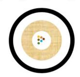
M3I-6M-R-BK fiber optic cable is constructed with six internal tight buffers, internal aramid yarn, and one outer riser-rated PVC jacket in distribution format. The cable is designed for indoor applications and features Corning ClearCurve® fiber.
