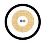
M4I-2M-P-BK fiber optic cable is constructed with two internal tight buffers, internal aramid yarn, and one outer plenum-rated PVC jacket in 900 $\mu$ m distribution format. The cable features a water-resistant jacket and is designed for indoor and outdoor applications.
